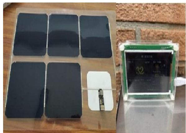
Fig.2: Solar panel and monitoring station
